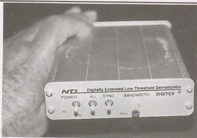
NTI Digitex digitally designed analogue threshold extension unit was created in Germany in two separate (non-compatible) modes - PAL or NTSC.
