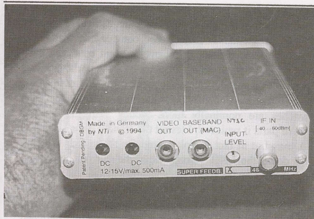
NTI Digitex digitally designed analogue threshold extension unit was created in Germany in two separate (non-compatible) modes - PAL or NTSC.
