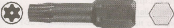
TORX tool has unique 6-spoke "wheel" with a centre-pin hole for accessing the Nokia innards.
