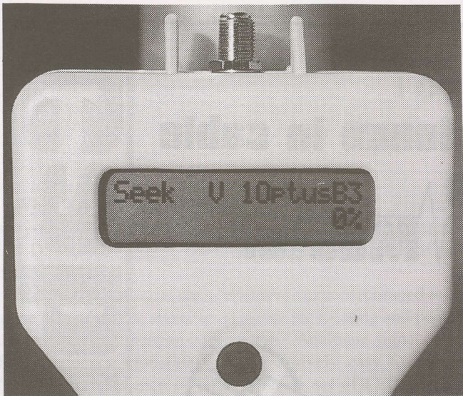
LCD readout is black against greyish tint display screen background - it is actually easier to read in bright sunlight than in a dimly lit room.
