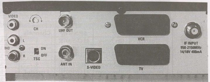
RCA sockets (left), PAL plug connections (next to right), SCART socket connectors and F fittings (right) are all susceptible to oxidation.
