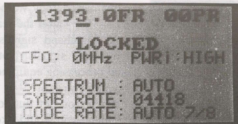
Spectral display on AsiaSat 3755/1395 (well, close) vertical - Arirang TV at centre. Set up for digital analysis (middle) shows CFO (signal centred in pass band) at 3757/1393 - see text. On right, Arirang "CH(annel) BER" is indicated 5.8E-3, Post Viterbi BER is 4.9E-5 and Reed-Solomon error count at time of photo was RU00005. See text.
