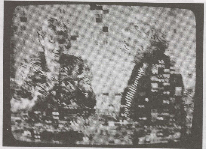
PIXELATION. Image locks, goes into squares and tiles at threshold point (above). BER indicator indicates point at which threshold is reached (below - installer menu readout from SA D9223).
