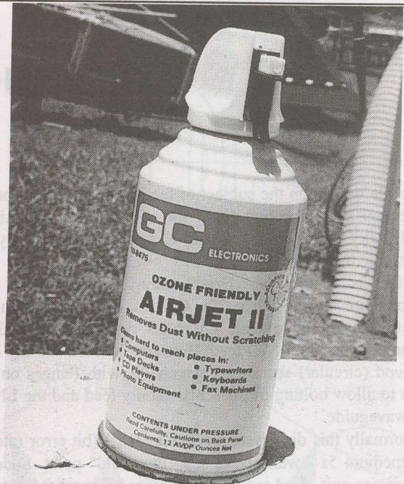
Compressed air (gas) in a can is good first level attempt for spiders and dead insects but if the mud is stuck to the walls, it won't work.
