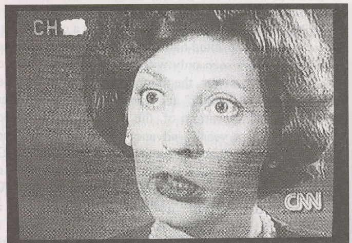
Totally different effect - same point in time, same cable system. Horizontal streaking created by imbalance in amplifier automatic gain circuits.
