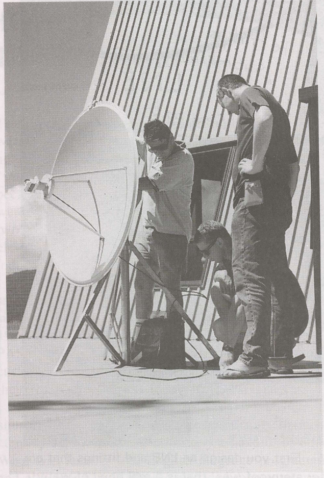
1.2m Paraclypse proving itself at 5 degree look angle on AsiaSat 2 services from European Bouquet
