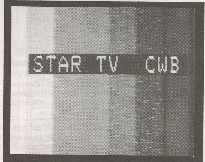
STAR TV UPLINK (CauseWay Bay-CWB) as it first turned on January 15 to test analogue uplink via AsiaSat 2. Photo from 2.1m dish at SatFACTS (NZ) with look angle near 5 degrees.
