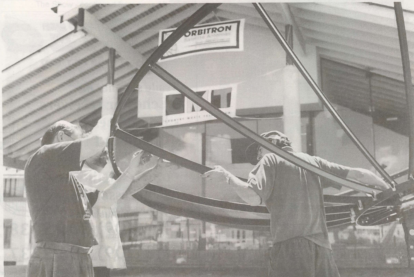
IT GETS EASIER EACH TIME. Bay Satellite's Stu McLeod, perhaps the most talented precision dish system assembler in New Zealand at the present time, knows that dish fine tuning begins with careful step by step assembly. McLeod's skills are second to none in setting a dish to full arc tracking.
