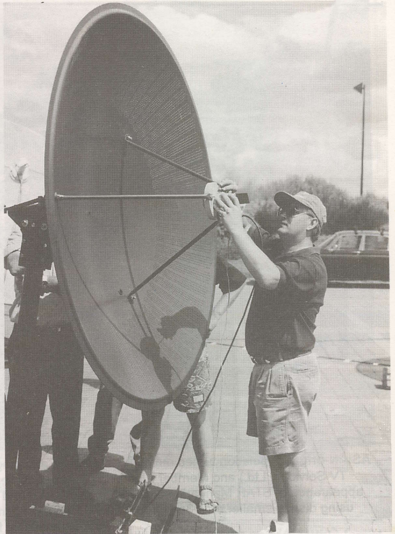
Paraclipse USA's Norm Bruner adjusts feed on Hydro 1.8m receiving AsiaSat 2 during SPRSCS '96
