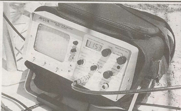
Analyser adjustments for earth noise measurements: (1) Slow scan rate speed way down, (2) Narrow scan width to as little as 1 MHz, (3) Use most sensitive scale (i.e., 2dB per division) linear display
