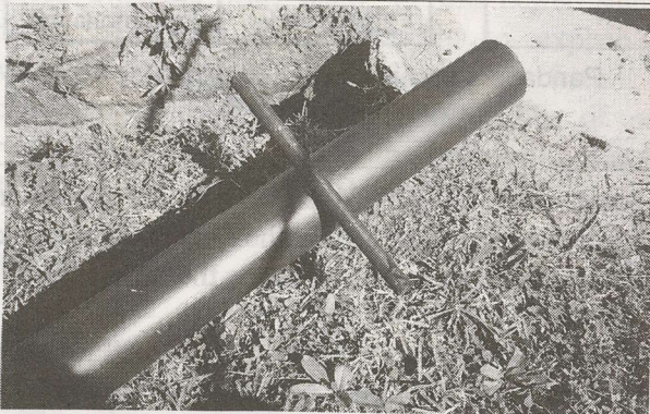
Schedule 80 steel pipe has crossways rod welded to it at approximately 1/2 the hole depth
