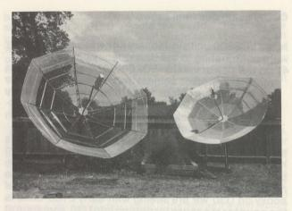
EXTENSION panels from SMP on 12 foot and 9 foot Paraclipse models. Wind and the strength of the mount are the main obstacles to a successful installation.
