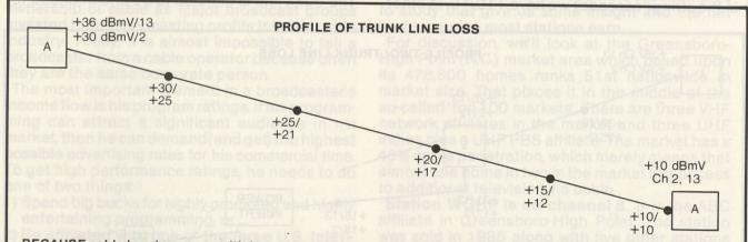
BECAUSE cable loss increases with frequency, the amplifier station operates with greater output level at channel 13 than at channel 2. This ratio (6 dB in example) closes along the pathway to the next amplifier 'flat'; +10 dBmV in our example.
