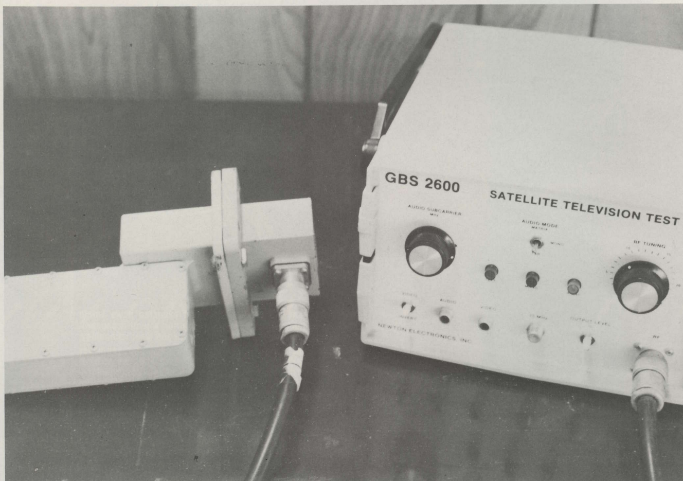
TEST SYSTEM consists of known signal input (source), controllable amounts of 4 GHz signal energy (ahead of and after LNA) and dedicated downconverter and receiver coupled to test monitor and/or spectrum analyzer.
