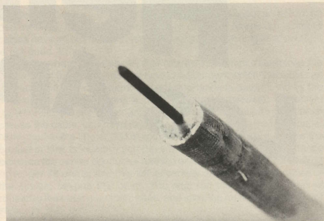
ALUMINUM JACKETED cable has solid aluminum sheath, an inner insulation of air bubbles and plastic (dielectric) and a center conductor of solid or copper coated aluminum.
