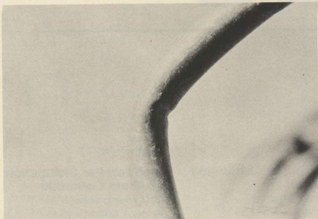
OOOPS! This piece of .412 cable got bent too tightly and the crease in the aluminum jacket will spoil the cable's performance.
