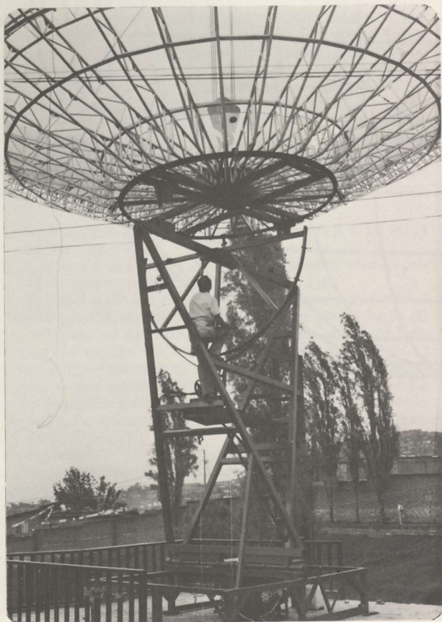
11 METER monster designed and constructed by Mario Yepes of Medellin, Colombia has what it takes to deliver at least five above-threshold video signals deep into Colombia, from F3R.
