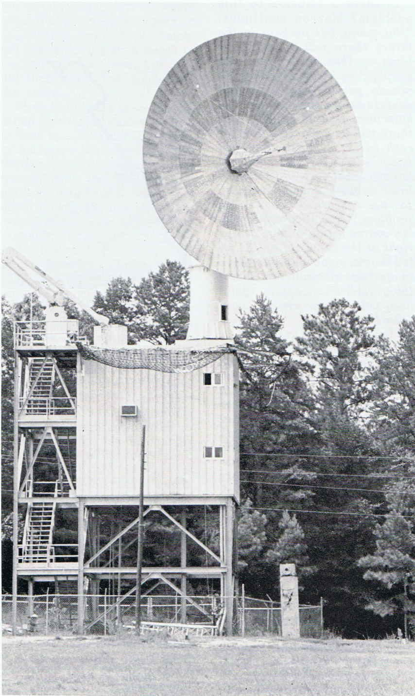
Aside from the elevated building structure housing the test range antenna measurement facility, this 10 meter dish could well be located at a CATV facility.
