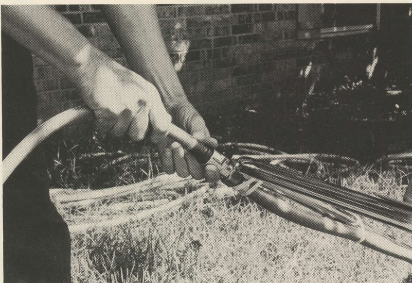
LUBRICATING WATER has a machine-mounted handle-valve to turn the water on as you start up the machine and begin the bore.
