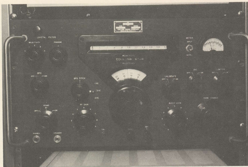
AUDIO SERVICES RECEIVER —a communications receiver (Collins 51J4 with product detector for single sideband here) plugged into the baseband output of a TVRO receiver is the essential 'additional ingredient' to adding audio reception to a TVRO receive site.
