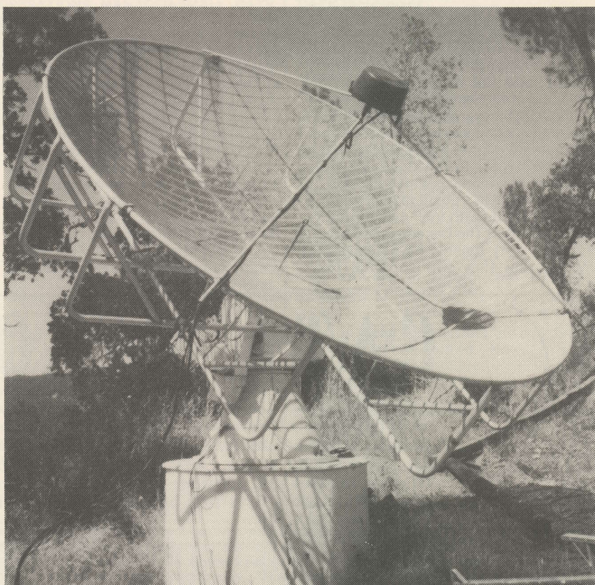
PRIVATE TERMINAL of California's H.T. Howard was constructed from surplus 4.5 meter radar antenna installation; surface is screen material originally utilized in a 150 foot aperture Stanford Radio Astronomy dish.
