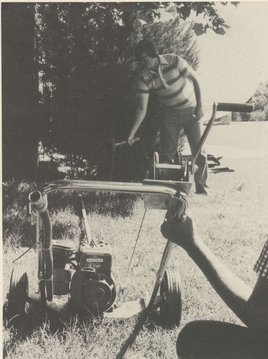
READY TO GO —the drill stem pipe is attached to the front coupling and the pipe aligned with hand driven rods that align with the exit hole intended.
