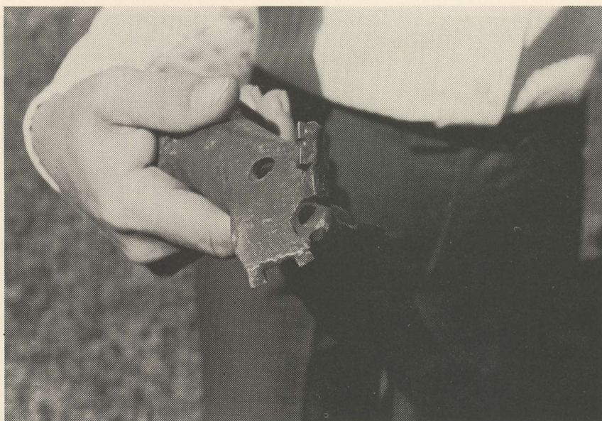
2.25 INCH BIT—three 'hungry teeth' and an exit hole that allows the lubricating water to exit the boring bit and force dirt back out of the hole to the rear.
