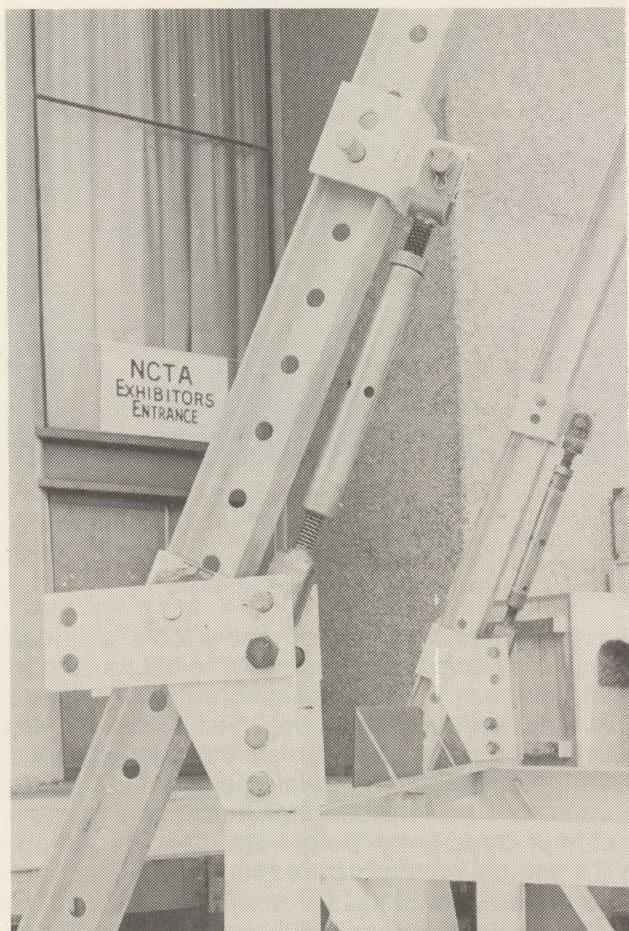
ELEVATION STRUTS on the SATRO-5M adjust the elevation; a pair of turnbuckle type screws provide fine adjustment on elevation.
