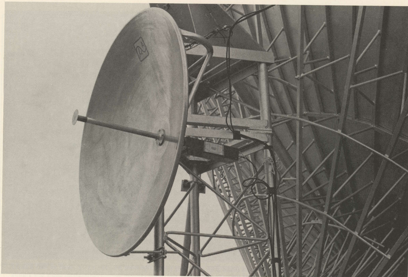
FOUR FOOT TRANSMIT dish from Microwave Associates is mated with low-cost microwave Gunnplexer transmitter which mounts directly to feed flange at rear end of dish antenna. Using this test system high quality video signals over paths as great as 20 miles proved practical under 'dry weather' conditions.
