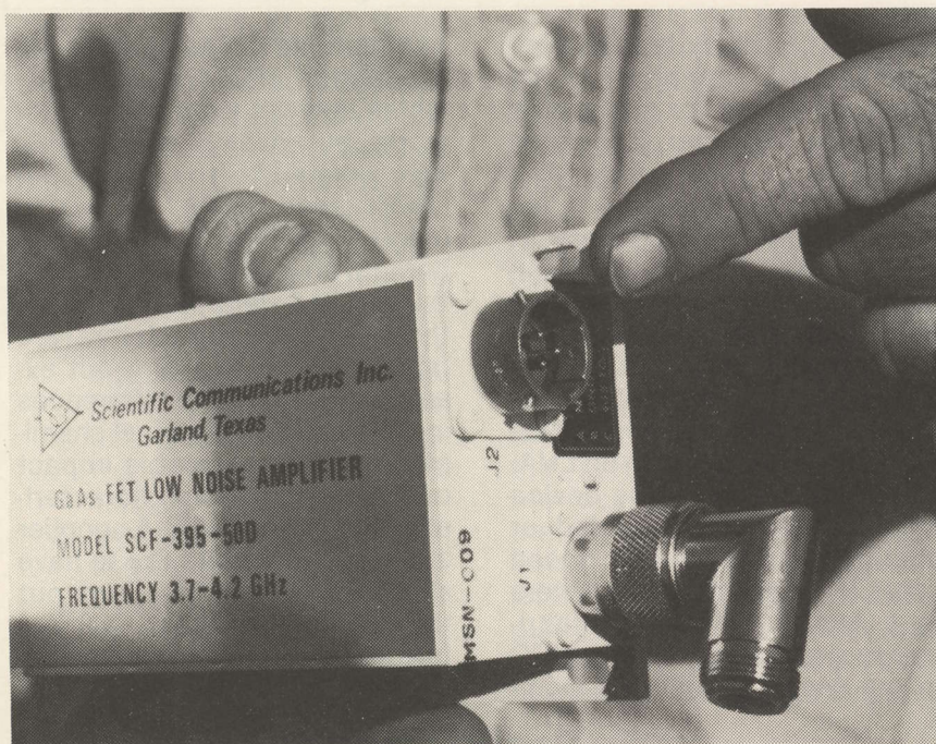
LNA AFT END pointing out operating power connector and right angle transition fitting to connect 'pigtail' patch line to 7/8ths downline for trip into CATV headend.
