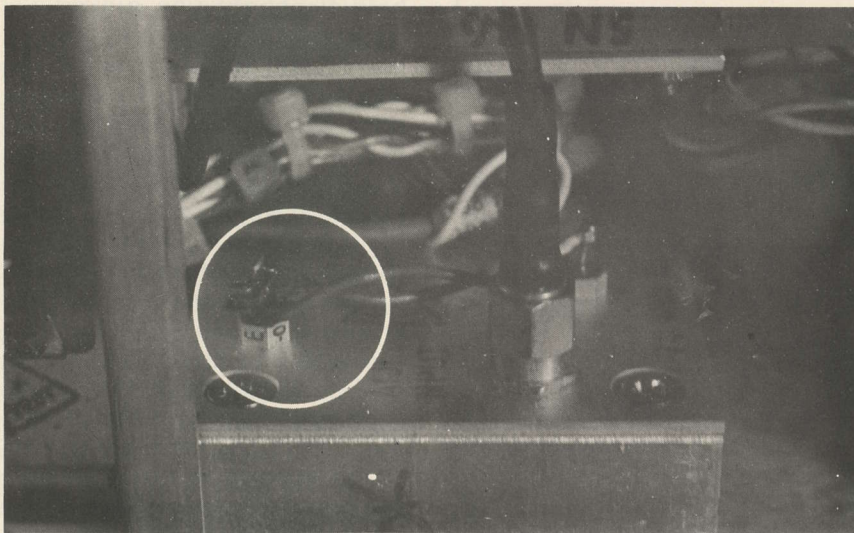
INSIDE RF TUNER MODULE/+15 volt line serves several separate sub-modules. Lines comes to and exits from feed-through chassis mounting capacitor (left, in circle) of 70 MHz gain control amplifier. Line must be removed from feed thru, tied back together to check sub-module.
