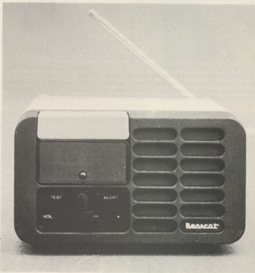
PROTO-TYPE CRYSTAL CONTROLLED receiver utilized during Anderson, Indiana tests proved effective but perhaps not decisively better than 'ho-hum' hand carried tuneable portable FM radio.
