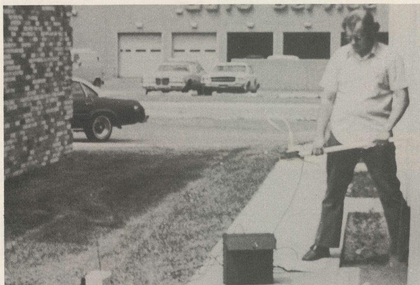
WITH RADIATION TEST SET you can play 'detective' and actually spot unauthorized second outlets (when done poorly) by patrolling the sidewalks and alleyways in an area. But watch out for dogs and angry people!
