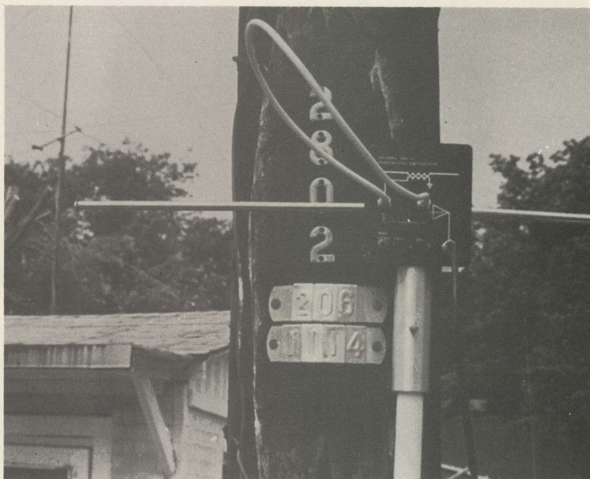
SEE GROUND WIRE coming down the pole? It confused the radiation level and source, acting as an 'unshielded transmission line' carrying the radiated signal down the pole (largely vertically polarized because of grounding wire polarization).
