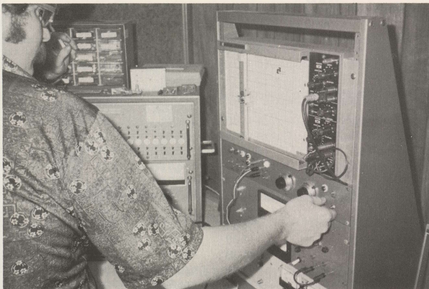
OPERATING PARAMETER PLOTTING with the HP "X"/"Y" plotter develops individual operating curves for single amplifier amplification devices, similar to those shown here for PT 4145 unit (versus B-022 device).
