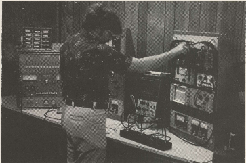
GAIN AND FLATNESS check on modified popular-brand amplifier under the careful direction of Chuck Wise.
