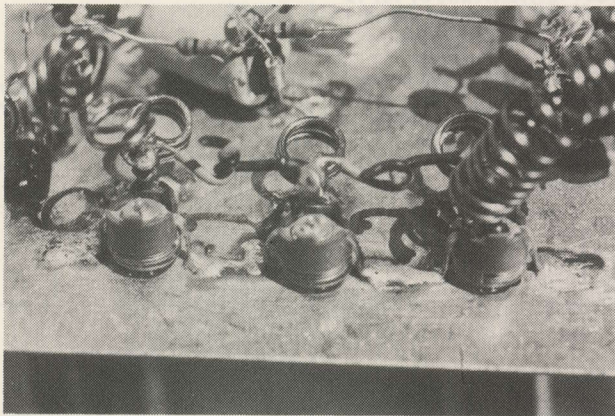
BANDPASS FILTER SECTION OF SWAN high band (channel 8) pre-amplifier fits between input and output amplification stages (see schematic and text).
