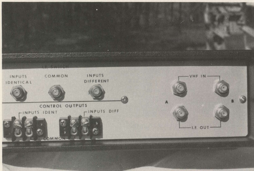
ADS-1000 SERIES switcher unit has host of inputs and I.F. inter-connection cable ports on back apron, as well as external control switching connections and time delay (optional) adjustment pot.
