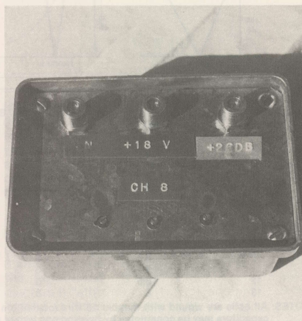
SWAN SINGLE CHANNEL PRE-AMP is housed in a readily available MATV type housing using locally fabricated sheet for bottom plate. Three adjustments along bottom are for bandpass filter section.
