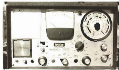
Texscan/Theta-Com Model 7270 SLM has new peak detector and 90 dB rotary attenuator in 10 dB steps.
