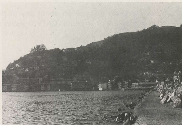
The South Sausalito setting is perfect for cable's basic master antenna function. The steep hill on the southside of the community blocks direct reception of San Francisco signals. Some signal escapes around and over the hilltop, but the pictures are severely degraded with multi-path ghosting.
