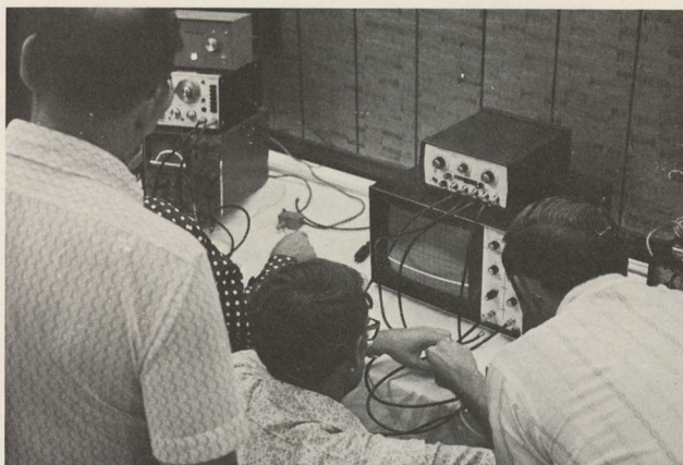
THANKS WAVETEK — with the kind loan of test gear by Bob Welsh of Wavetek, the CCOS Lab Room proved a very popular and innovative feature of CCOS. Small box atop stack at left is Richey's July 1974 CATJ Mark-A-Channel construction project; here in use to mark video and audio carriers positions on bandpass filter being aligned on test station to left.
