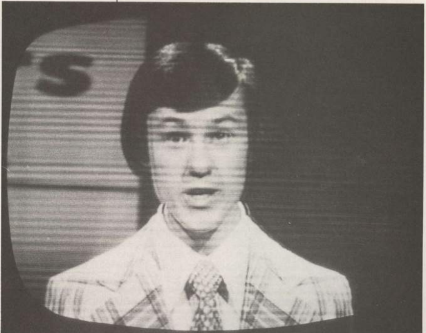
20 dB DOWN AND 20 kHz — A precision 20 kHz offset carrier generated in the CATJ Lab is beat against an off-air broadcast signal; at an interference level 20 dB below the off-air signal, to produce this photograph. Thirty-three similar co-channel photos are displayed in CATJ's new FCC Tests Wall Chart.
