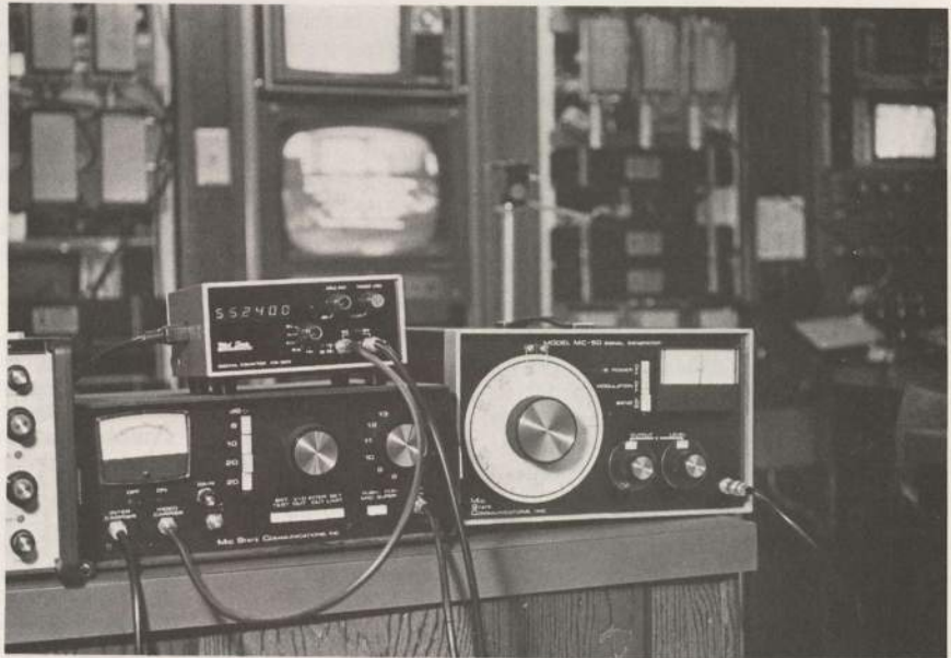
CREATING CO-CHANNEL — Interfering carrier generation equipment (MC-50) with a portion of the frequency (and level) monitoring equipment employed to prepare CATJ FCC Tests Wall Chart.
