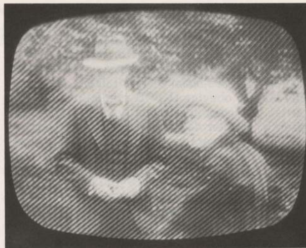
HARMONIC CREATES HERRINGBONE BEAT —Harmonic signal falling into TV channel 2 creates herringbone "film" over picture; ratio of harmonic signal level to channel 2 signal level determines "degree of blanking" of TV picture.
