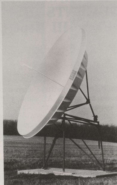
PRODELIN 15 FOOTER — One of several existing 15 foot (give or take a foot) earth terminal antennas is the Prodelin Masar model.
