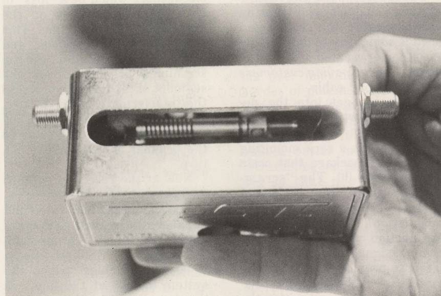
"DESCRAMBLER" ALA T.E.S.T. — Special Dallas show unit had cut-away for view inside of glass and ceramic substrate of trap unit.
