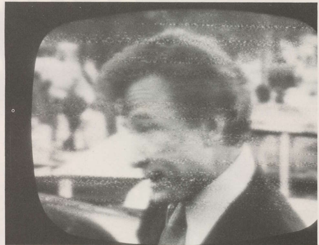
MOTOR NOISE/LOW BAND — Noise peaks average 25 dB below visual carrier level.
