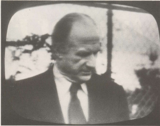
MOTOR NOISE/LOW BAND — Noise peaks average 35 dB below visual carrier level; note start of noise-banding along extreme bottom of screen.
