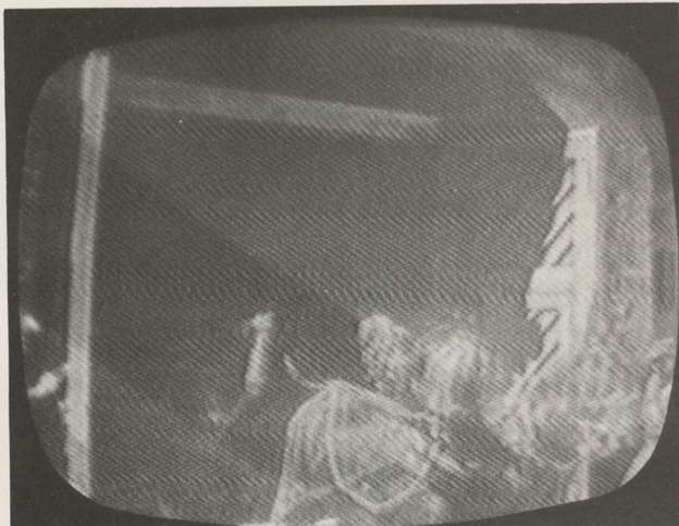
10 ADJACENT TO 9 — With 10 visual down 15 dB (9 aural herringbone degrading)
