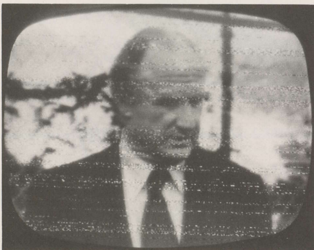
MOTOR NOISE/LOW BAND — Noise peaks average 20 dB below visual carrier level.
