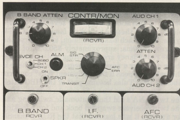
Top-portion TerraCom receiver with meter-reading functions and controls.
