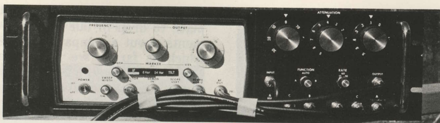
WAVETEK 1051 TEST SET — standard 1051, modified for factory rack mount, addition of "tilt," with addition of test set attenuators, switching and comparators discussed in text.
