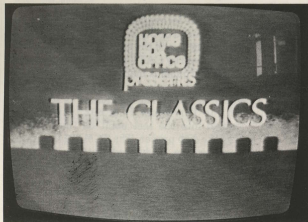
HBO identification and introduction to feature film; photo taken from 25 inch color receiver in Tulsa Cable lobby, picture showed noticeable degradation from video monitors in headend.
