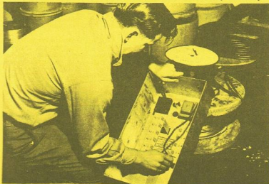
Fig. 8. Wiring an ADO-10 antenna distribution box for use in the Panther Valley "community aerial" system. Signals from Philadelphia's three television stations, seventy airline miles away, are being received in Lansford, Pa., clearly and cleanly.
