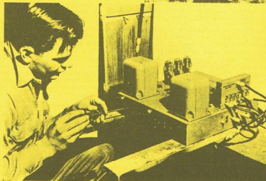
Fig. 6. A "PV-TV" technician adjusts a new MC-1 master control and amplifier unit before installation. The unit amplifies each channel separately and then mixes the amplified television signals in the output to system's distribution boxes.
