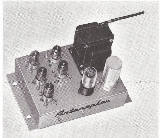
Broadband Amplifier, MI-5301 (with cover removed)
