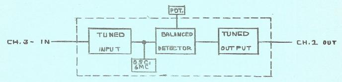
The converter output may contain a Channel 4 component, which is highly attenuated with respect to the desired Channel 2 output. It may be desirable to further attenuate the Channel 4 signal before feeding to an AGC amplifier which operates with Channels 2, 4 and 6 in the output mixing network. Removal of spurious Channel 4 signal is accomplished by inserting an open quarter wavelength coax stub in the output line from the converter, as follows:
