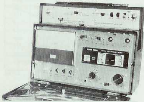
BLONDER-TONGUE FSM-2 with auxiliary sub-band converter covers through 83
